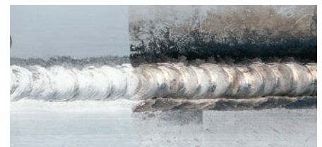
Example of the action of BOC Weld-Guard™ Aluminium Pickling Gel.
