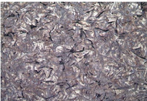
Microstructure of grey cast iron (x200)
